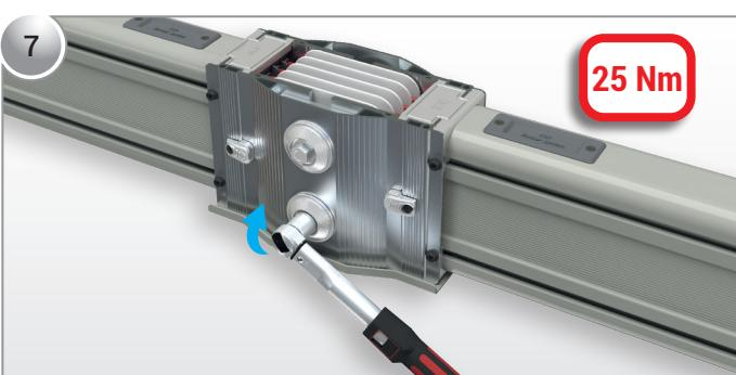
Reinstall the nut locking covers and torque with 25 Nm.
