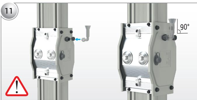
Open the plastic cover on the opposite side of the block joint to be cast, and install the CCR-II Block Joint Casting Level Control Plastic.
