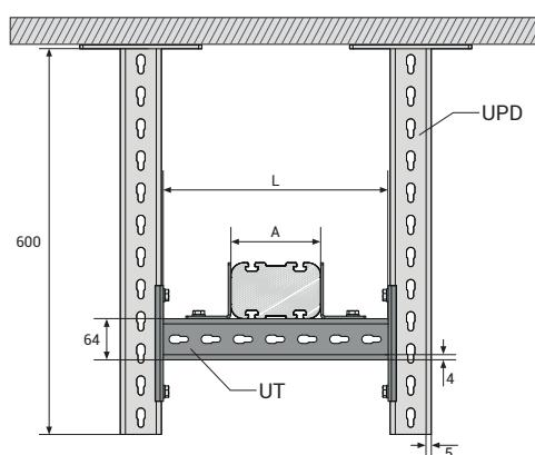
When choosing CCR-II-UT Suspension Set, appropriate CCR-II-UT Suspension Set should be selected according to Busbar size.
