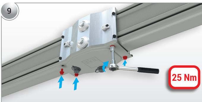
Torque the bolts of the lower block joint cover to 25 Nm.
