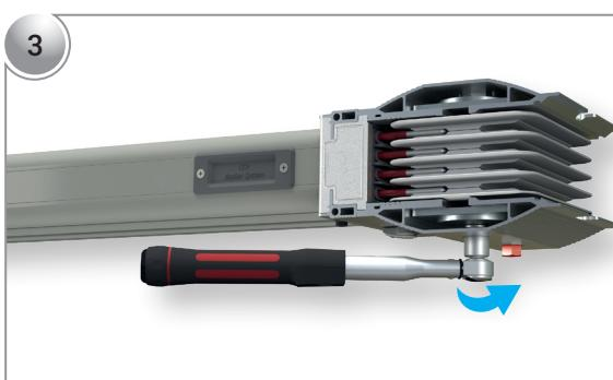
Loosen the block splice nuts.
