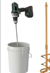
Mix the mixture with a beater at low speed for at least 30sec - 1 minutes until it is homogeneous.
