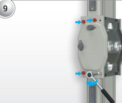
Install the other block joint cover and torque its bolts to 25 Nm.
