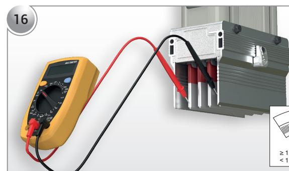
An insulation resistance test must be conducted at least 24 hours after the procedure is completed.
