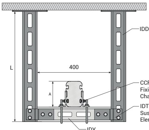
**!** When selecting IDD products, the appropriate IDD product should be selected based on Busbar A measurement.
