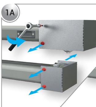
Remove the busbar protection covers by unscrewing the bolts
