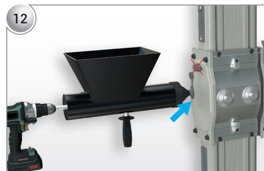
Inject material through the filling hole as shown. Continue filling until Flex-Comp is visible inside the level control plastic.
