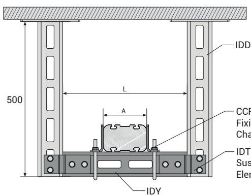
**!** When selecting IDY products, the appropriate IDY product should be selected based on Busbar A measurement.
