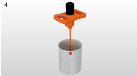
4 Mix resin and hardener thoroughly with stirrer at least 30-60 seconds.
