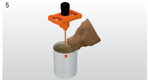
5 Add fillers and mix until homogeneous; at least 2-3 minutes. Then application must be done within 15 minutes.
