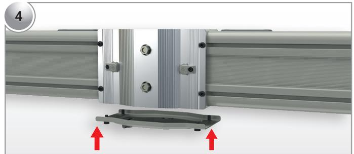
The joint block cover is attached to align the block joint and the bolts are tightened not too strong.
