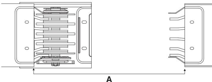
Measure "A" length in cm, to determine the length of special busbar subtract 12 from "A".
