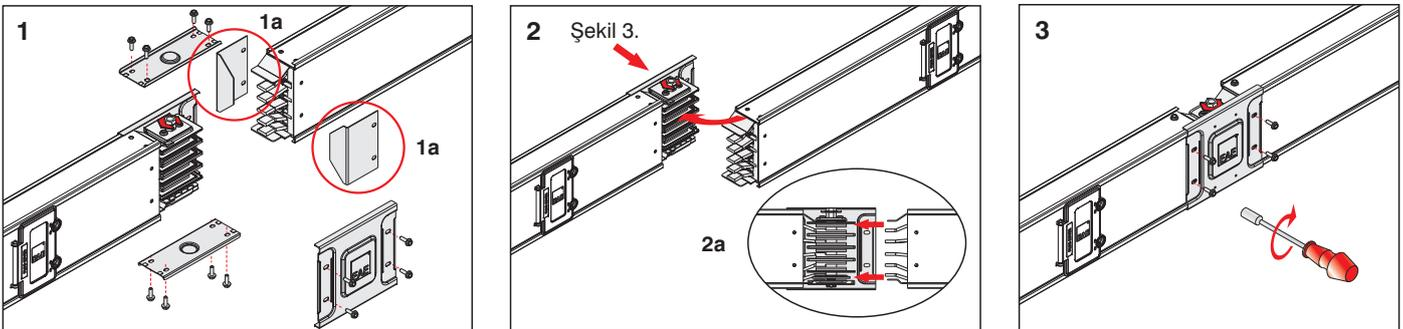
1- Remove joint top cover plate, joint side cover plate and the screws from non-block joint bolt. (Pieces marked as 1a should be thrown away.)
