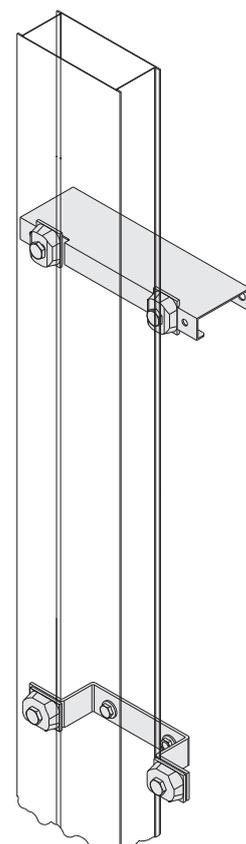
■ The span between supports should be 1.5m
