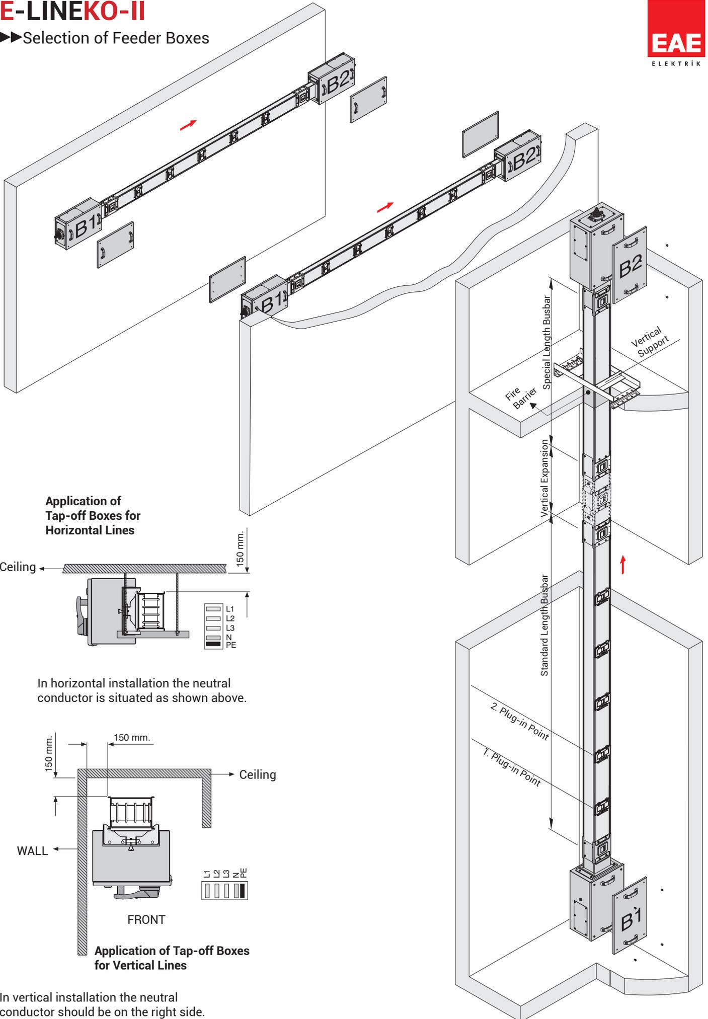
In vertical installation the neutral conductor should be on the right side. It is important for tap-off box connections.
