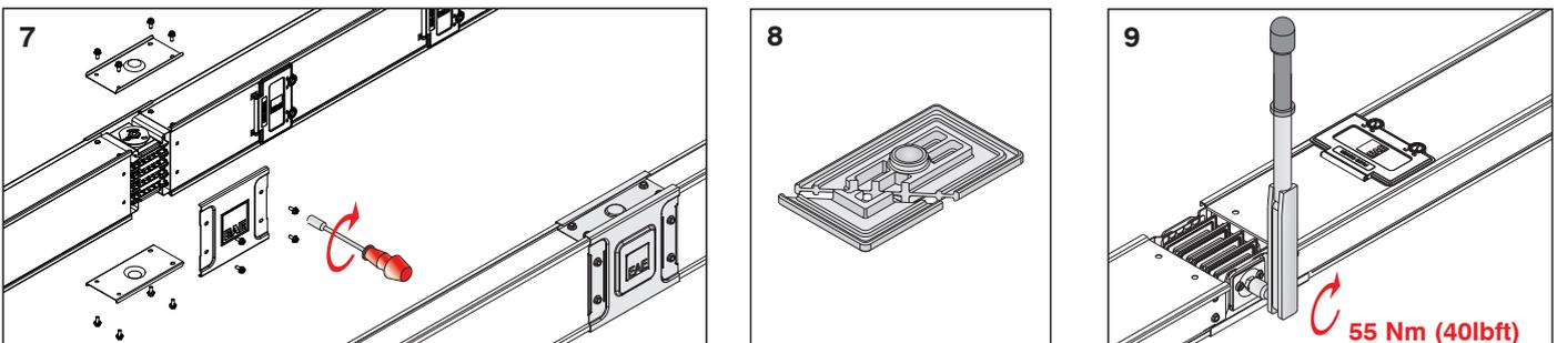
7- Install top and bottom joint cover plates. Check the joint before fitting the last joint side cover plate. Fit the joint cover side plate and tighten the screws. Check the position of the earth conductor when installing KO-II with five conductors.
