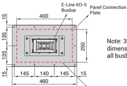
Note: 300x460mm flange plate dimensions are standard for all busbar types.
