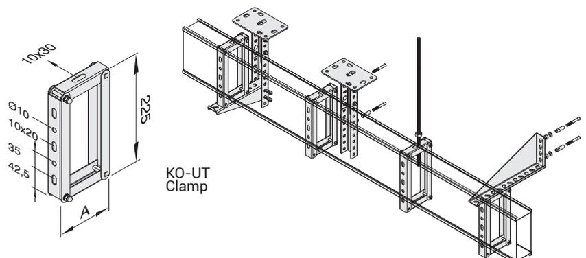
■ The span between supports should be 1.5m
