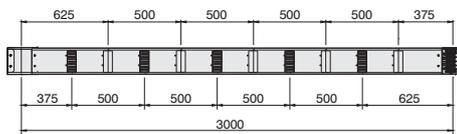
Electrical Power up to 400A can be supplied from the busbar by Tap-off boxes.
