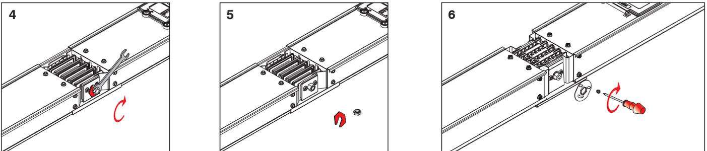
4- Tighten the double headed nut until upper nut is broken.
