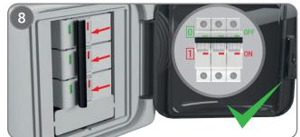
Switch miniature circuit breaker (MCB) to "ON" position and close the transparent cover.
