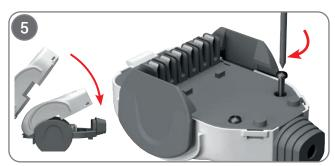
Replace the plug cover, turn the plug upside down and replace the two screws on the back.
