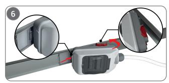
Open the closed plug-in opening on the busbar. The insertion direction of the box should be as shown in the figure. Tabs which located on the edge of the tap off box must be installed to the current output windows which located on busbar itself with an angular position. Tap off box should be positioned parallel to the busbar.
