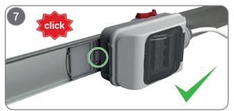
Spring type parts which located on the edges of the tap off box should be installed by pressing to the busbar by making sure of its totally merged.
