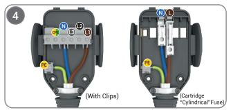
Please connect the yellow/green protective conductor to the earthing (PE) terminal, the blue neutral conductor cable to the neutral (N) terminal, and the other phase cable(s) to the relevant phase (L1, L2, L3) terminals. (Caution: Make sure that the terminal screws are tightened enough.)
