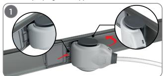
Open the closed plug-in opening cover on the busbar. The tap off plug should be installed in the direction as stated in the figure. Tabs which located on the edge of the tap off plug must be installed to the current output windows which located on busbar itself with an angular position. Tap off plug should be positioned parallel to the busbar.
